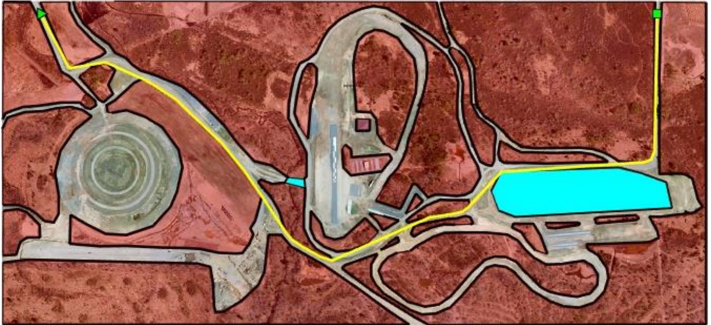
Figure 14 Planned path along the road networks and major drivable area at KRC with a washed-out bridge and flooded zone (light blue) at 4 inches of rain per hour.
