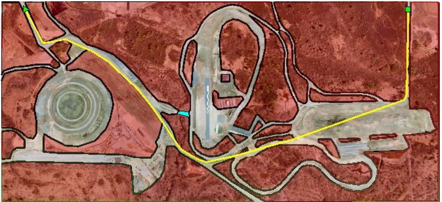
Figure 13: Planned path along the road networks and major drivable area at KRC with a washed-out bridge (light blue) at 2 inches of rain per hour.
