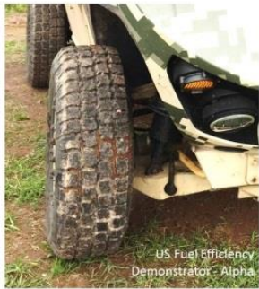
Figure 5: Detail of the FED-A tire pattern and soil impression.
