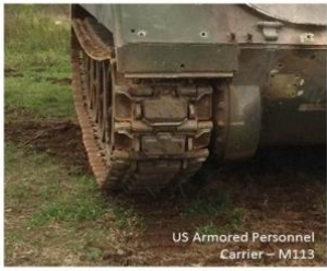
Figure 4: Detail of the M-113 tracks and soil impression.
