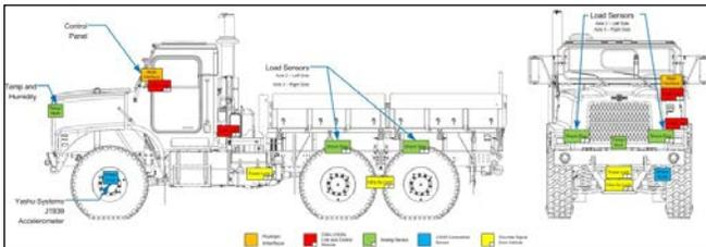
**Figure 3:** GS Engineering CTIS Control Module – Sensor Integration on MTVR
