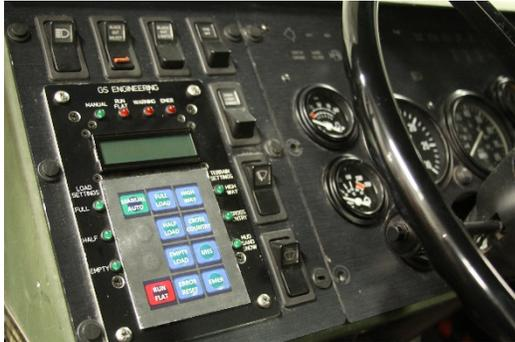
**Figure 2:** GS Engineering ACTIS Control Module User Interfaces
