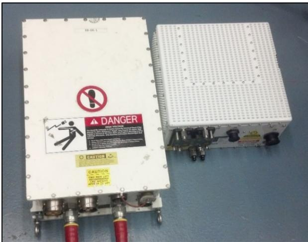
**Figure 3:** Silicon Converter (left) vs. SiC Converter
