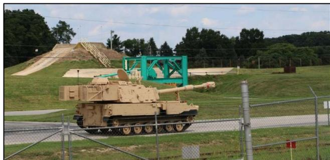
**Figure 9:** The M109A7 with Installed SiC Converter Driving on the Test Track
