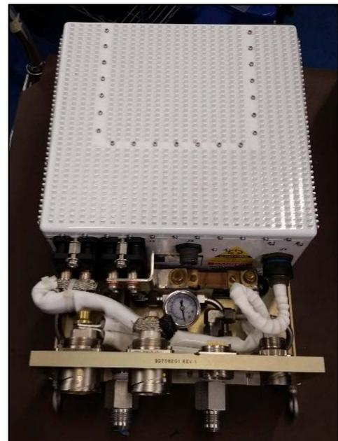
**Figure 4:** SiC Converter in Vehicle Fixture
