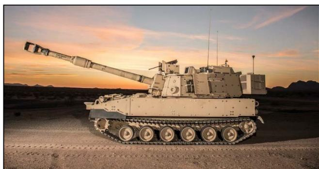
**Figure 1:** The M109A7 Self-Propelled Howitzer
