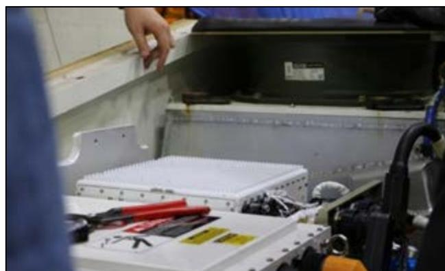
**Figure 8:** GE SiC converter in place of two BIDI's
