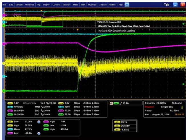
Figure 5: Transient Load Performance; 0 A to 400 A step
