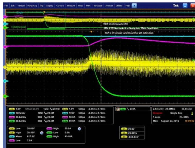
Figure 6: Transient Load Performance; 400 A to 0 A step
