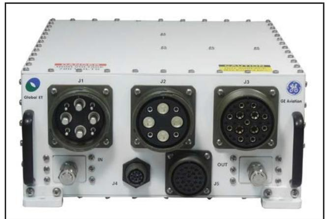
**Figure 5:** High Voltage Power Controller
