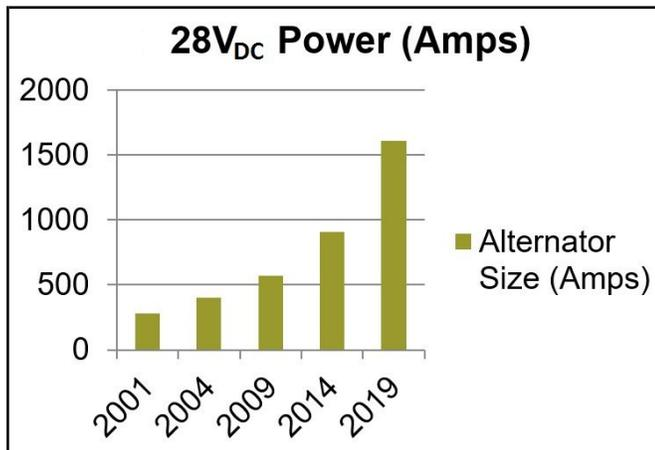
**Figure 1:** 28VDC Vehicle Power Demand
