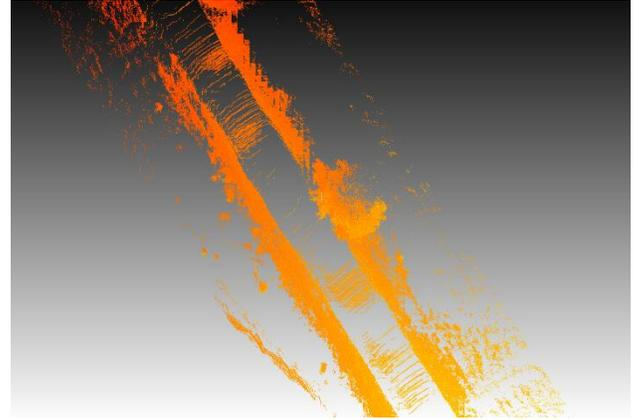
Figure 14: Union of all segmented obstacles with no terrain-sharing. Note the many mis-classified obstacles present in the roadway. The tree is present near the middle of the plot.
