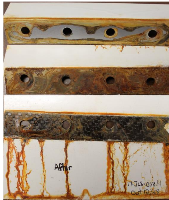
Figure 6: Galvanic assembly without adhesive disassembled after 1000 hours B117 salt spray to investigate substrate corrosion.
