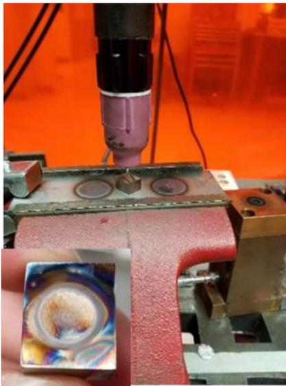
**Figure 3:** GTA spot welding set up with an image of the sample spot weld in the lower left corner
