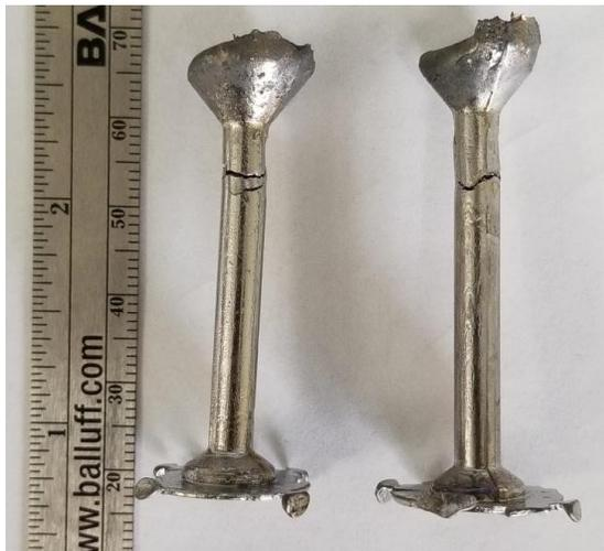
Figure 11: Examples of cracking in 1.375 inch and 1.5 inch cast pin
