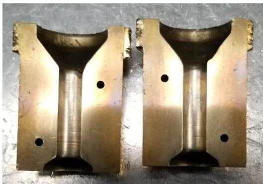
Figure 5: Example of CPTT pin mold
