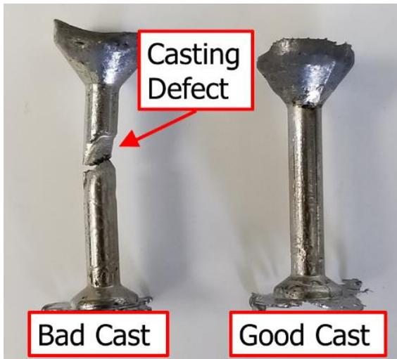
**Figure 8:** Image of two sample 1 inch pins. One pin exhibits cracking due to a casting defect, and the other is an ideal cast pin.
