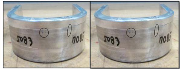
Figure 9: AA5083-H131 to AA7085-T721 bends test results at a) 120 and b) 110 rpm.
