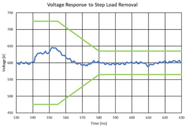
**Figure 6:** Generator Controller Voltage for 40 kW Load Drop Transient
