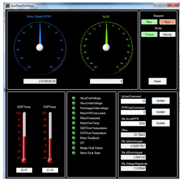
**Figure 2:** Generator Controller PC Interface Screenshot
