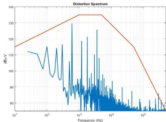
**Figure 8:** Generator Controller Output DC Voltage Distortion Spectrum
