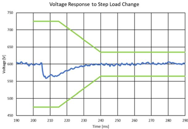
**Figure 5:** Generator Controller Voltage for 40 kW Step-Load Transient
