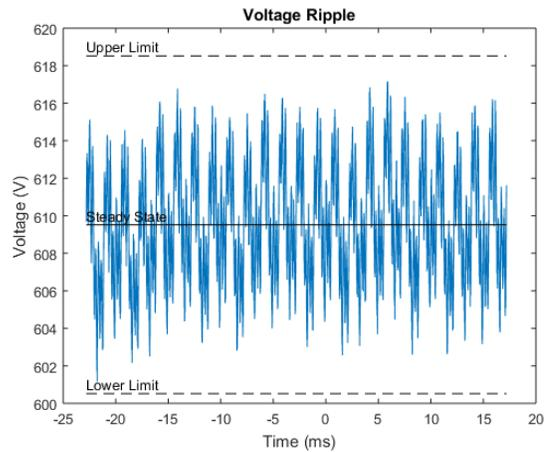
**Figure 7:** Generator Controller Output DC Voltage Ripple
