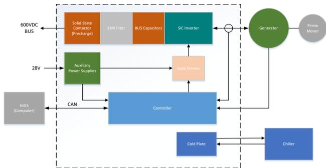
**Figure 1:** Generator Controller Functional Block Diagram
