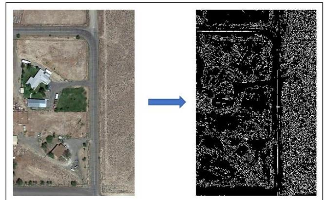
Figure 3. Canny Edge Detection on Satellite Map.
