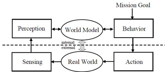
**Figure 5:** The fundamental structure of a 4D/RCS control loop. An internal world model of the external world provides support to both perception and behavior. Sensors measure properties of the external world. Perception extracts the information necessary to keep the world model current and accurate from the sensory data stream. Behavior uses the world model to decompose goals into appropriate action.
