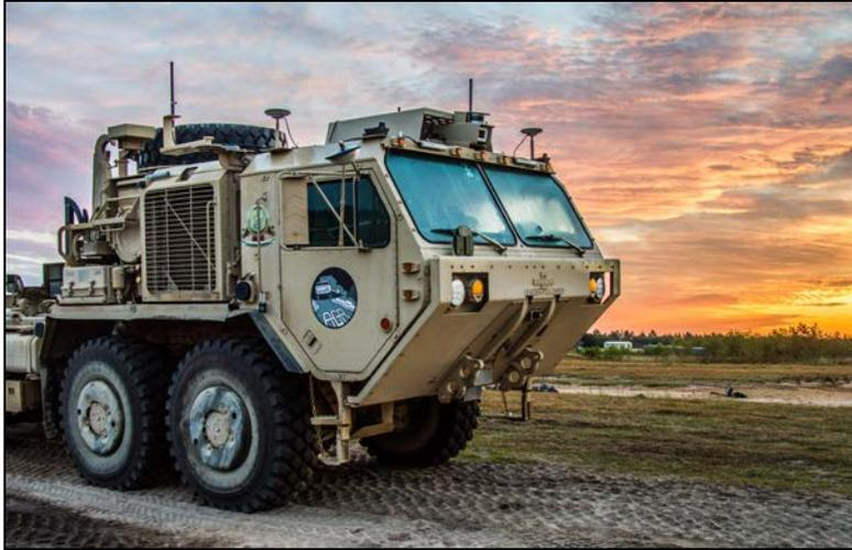
**Figure 1:** AGR SO system integrated onto PLS M1075A1
