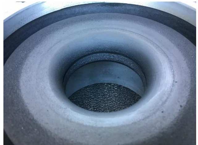
Figure 10: Coated compressor housing after service
