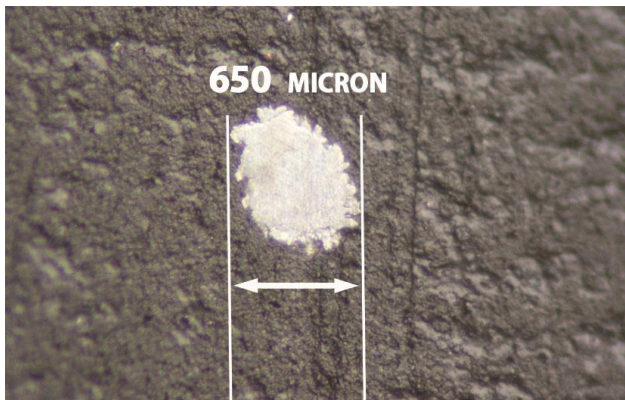
Figure 5A: Free Aluminum particle safely smashed and embedded in Slick+ AAPC piston skirt coating
