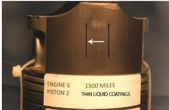
Figure 3A: Thin coating with normal IPWC. Narrow contact area, foreign particle scratches visible
