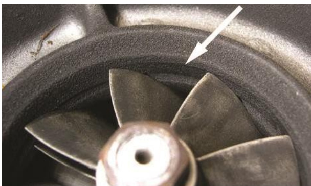
Figure 8: Rotor bedded into soft coating - perfect seal (zero clearance and zero friction) after 150,000 miles
