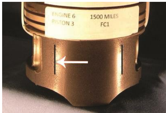
Figure 3B: Stribeck Fitting Results, Armor AAPC; reduced IPWC, larger contact area, extended oil leak path, reduced peak stress on oil film, limited rocking room, nearly scratch free while running alongside Figure 3A piston
