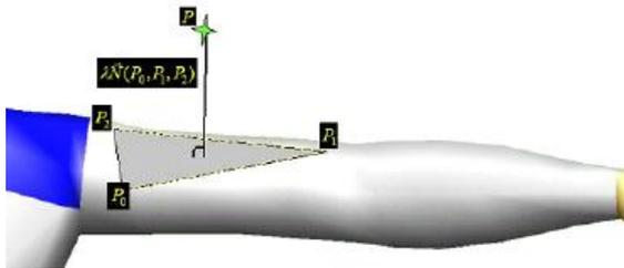
**Figure 2:** Definition of a reference point referred to the upper arm of a RAMSIS manikin
