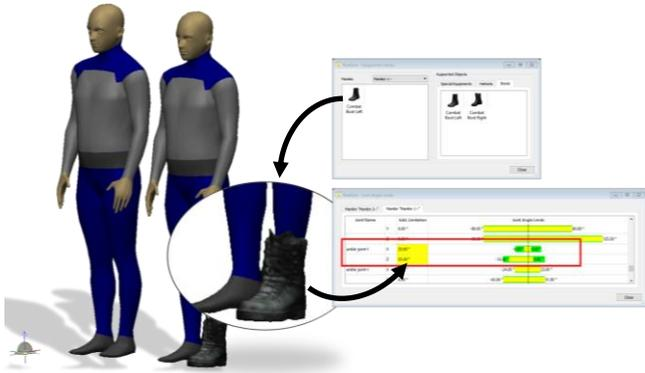
**Figure 6:** Manikin with attached boot from the equipment library to the left foot. Table with information on the limited ROM for flexion/ extension and pronation/ supination of the left ankle is displayed.
