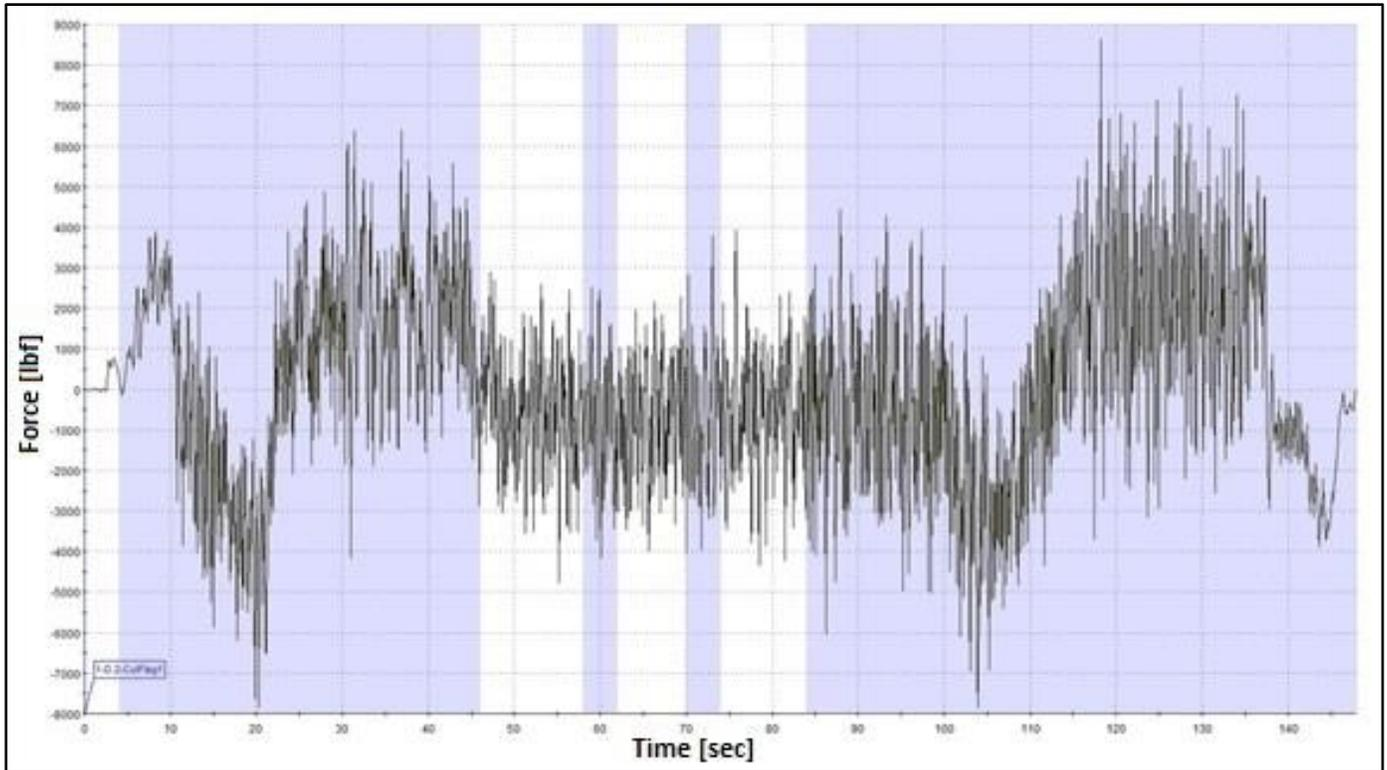
Figure 5. Example of file region selection based on fatigue damage.
