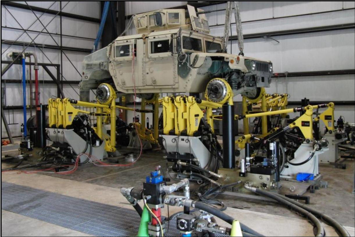
Figure 1. Up-armored HMMWV testing on the ATC VDS.
