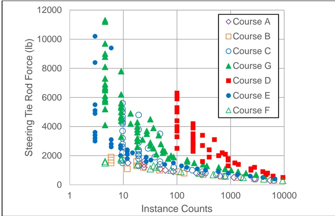
Figure 3. Rainflow analysis example of steering tie rod force data, for 10 miles on each test course.
