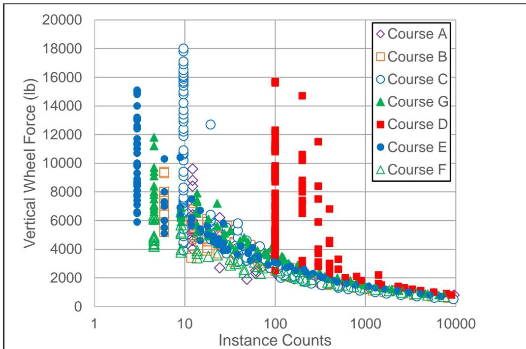
Figure 2. Rainflow analysis example of vertical wheel force data, for 10 miles on each test course.
