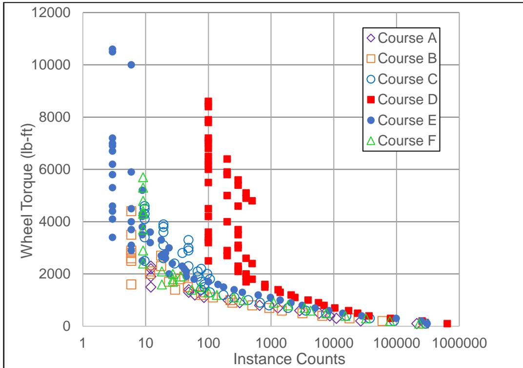
Figure 4. Rainflow analysis example of wheel torque data, for 10 miles on each test course.
