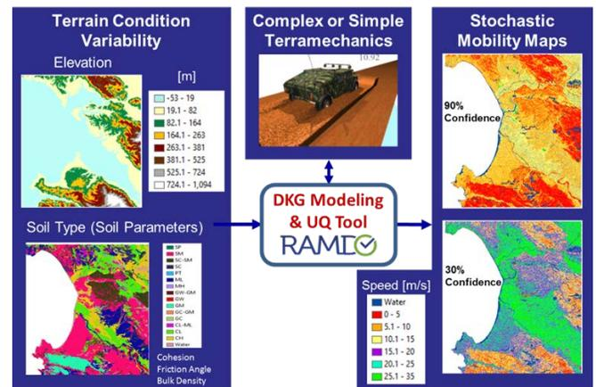
Figure 7. Propagation of Variability to Generate Reliability-Based Stochastic Mobility Maps
