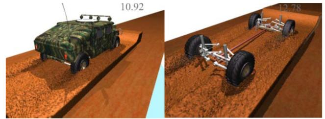
Figure 6. Complex Terramechanics Model of NATC Wheeled Vehicle Platform
