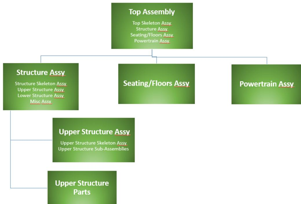
Figure 6: Sample Assembly Structure for the ACV
