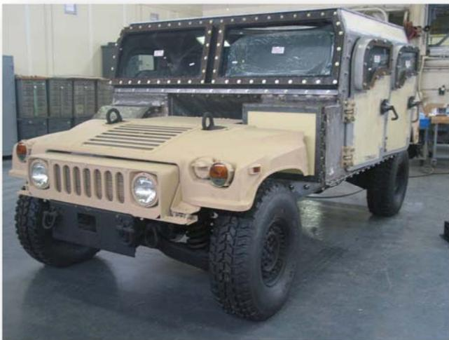
**Figure 3: HMMWV Improvement Program (HIP) Double V Hull Survivability Demonstrator**
