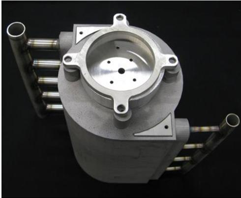
**Figure 3:** Picture of the 3D metallic printed (DMLS) Swiss-roll reformer.
