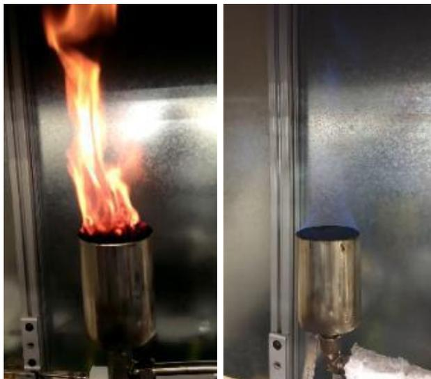
**Figure 10:** Reformat flare color. Left: Without mixing chamber. Right: With mixing chamber.
