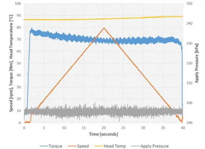
**Figure 10:** Speed Sweep of Non-LS Oil-Cycle 5
