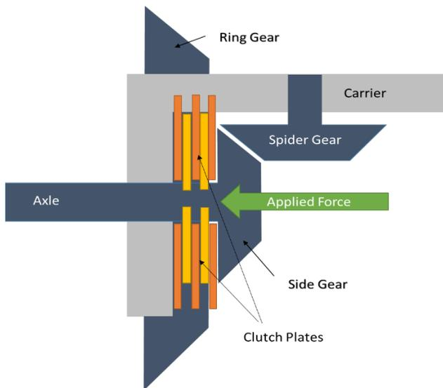
**Figure 1:** Cross-Section of Limited Slip Differential
