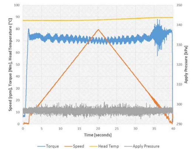
**Figure 11:** Speed Sweep of Non-LS Oil-Cycle 65
