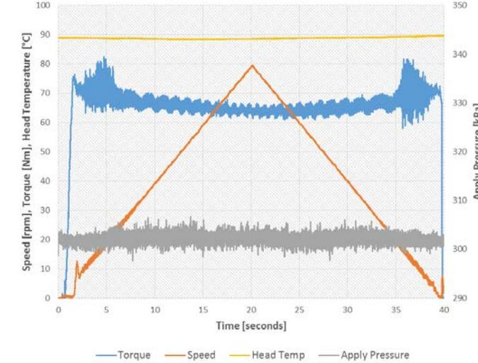
Figure 8: Speed Sweep of “Poor” Reference Oil-Cycle 25
