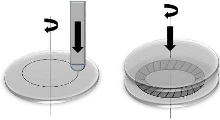
**Figure 3:** Pin-on-disc and Disc-on-disc Bench Test Configuration
