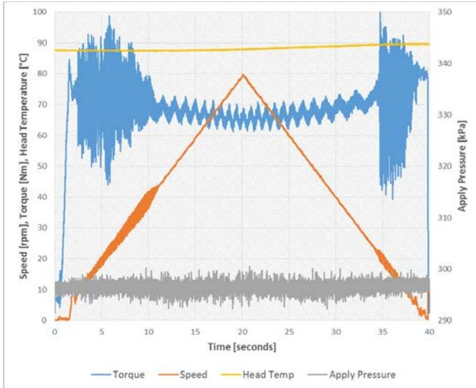
**Figure 12:** Speed Sweep of Non-LS Oil-Cycle 89
