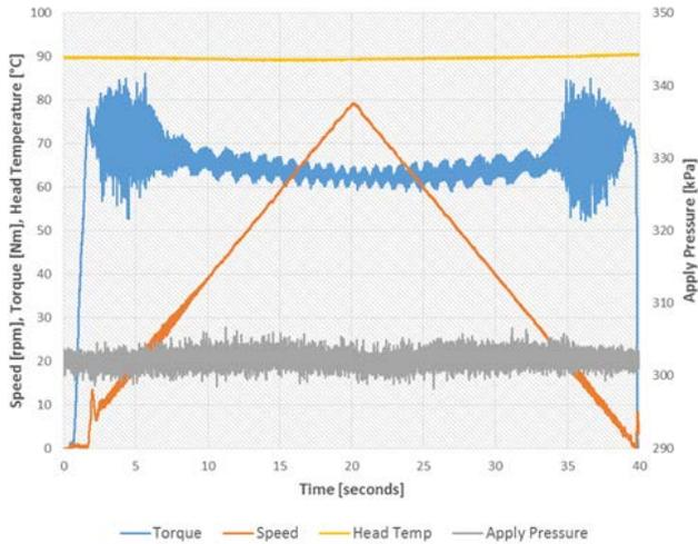
**Figure 9:** Speed Sweep of “Poor” Reference Oil-Cycle 50
