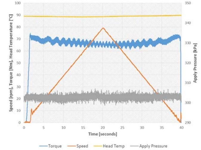
Figure 7: Speed Sweep of “Poor” Reference Oil-Cycle 5
