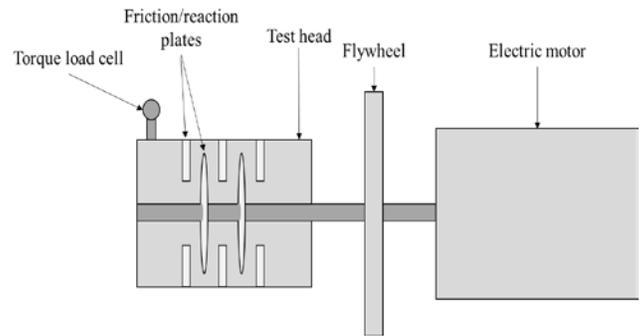
**Figure 2:** Basic Components of an SAE No. 2 Friction Test Machine
