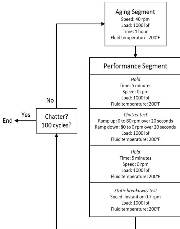
Figure 4: Schematic of the Proposed LSD Oil Compatibility Test Method
