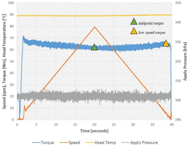
Figure 5: Speed Sweep of “Good” Reference Oil-Cycle 5
