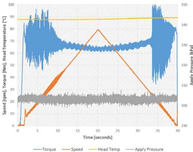
**Figure 15:** Speed Sweep of Top-Tier 75W-90-Cycle 16
