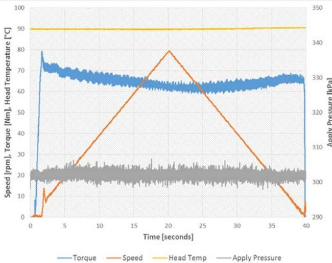
Figure 6: Speed Sweep of “Good” Reference Oil-Cycle 50
