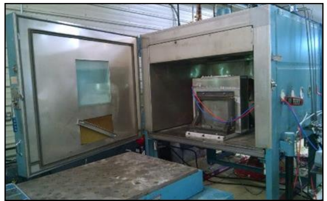
Figure 7: GLSV environmental and leakage test setup
