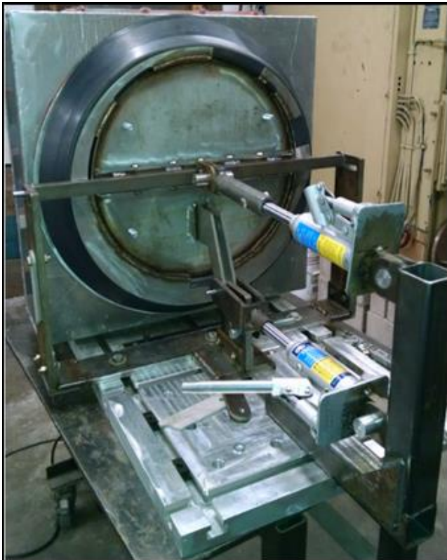
Figure 6: GLSV leak test fixture
