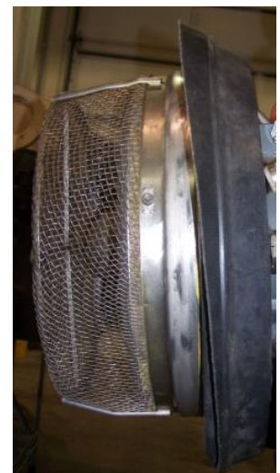
Figure 1: Plenum seal and FOD screen
