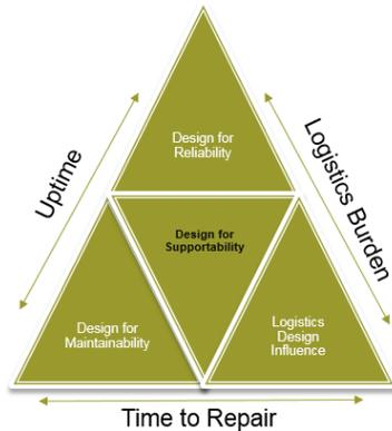
**Figure 2:** Relationship between Design for Reliability, Design for Maintainability and Design for Logistics
