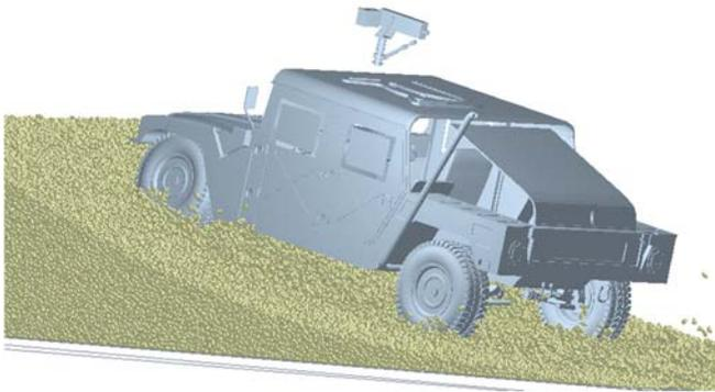
**Figure 7. HMMWV on single hill at 20kph**
