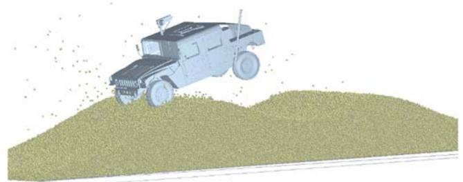
**Figure 8. HMMWV on double hill at 60kph**
