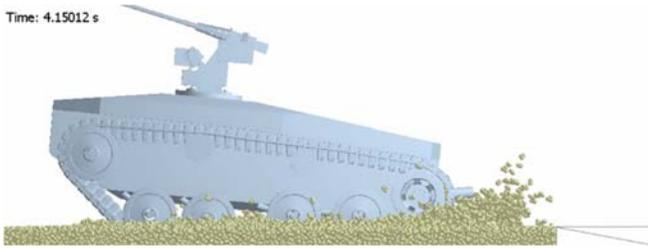
**Figure 15. Tank drawbar pull**
