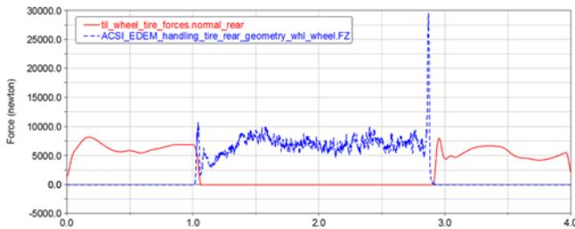
**Figure 17. HMMWV tire and particle forces**
