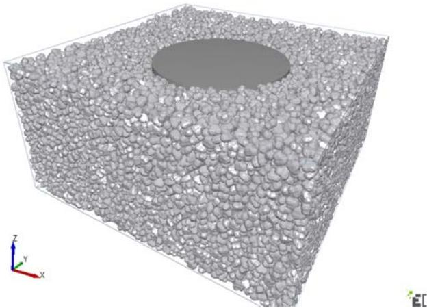
**Figure 21. Adams-EDEM testrig for soil parameter characterization**
