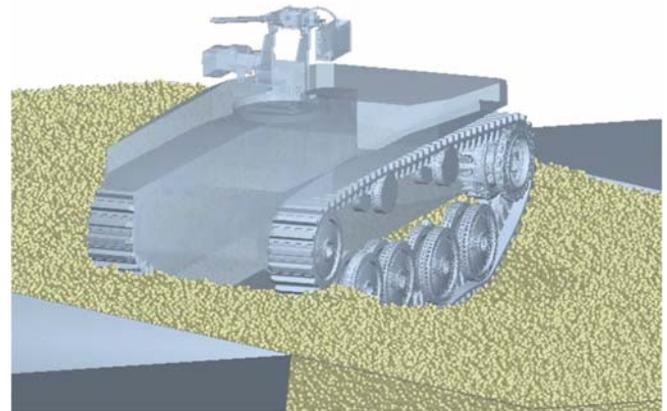
**Figure 14. Tank pivot-steer at 3kph, with opposite left/right track speeds**
