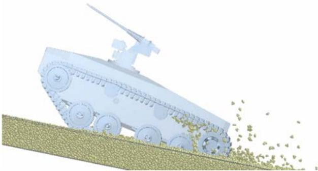
**Figure 13. Tank on 20pct grade climb, full throttle**
