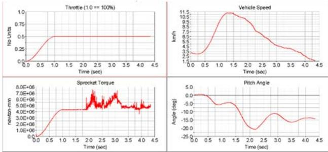
**Figure 19. Tank on 20% grade at 50% throttle**
