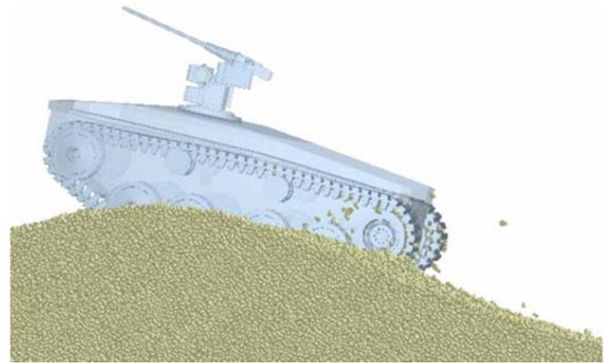
**Figure 11. Tank at 7kph becoming stuck on hill**
