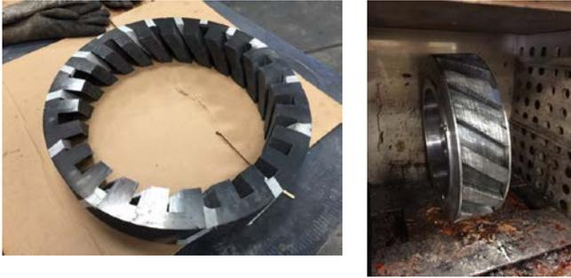
**Figure 8:** Stator and rotor development of the ISG.
