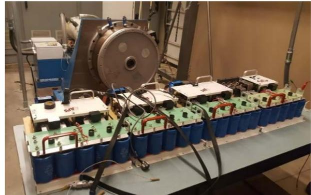
**Figure 11:** ISG Drive hardware placed on a dynamometer.
