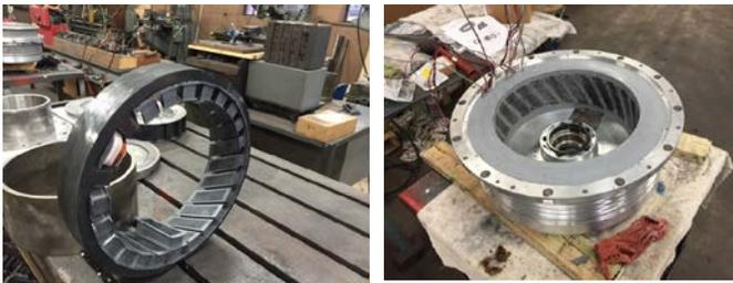
**Figure 9:** Stator assembly placed in the housing.
