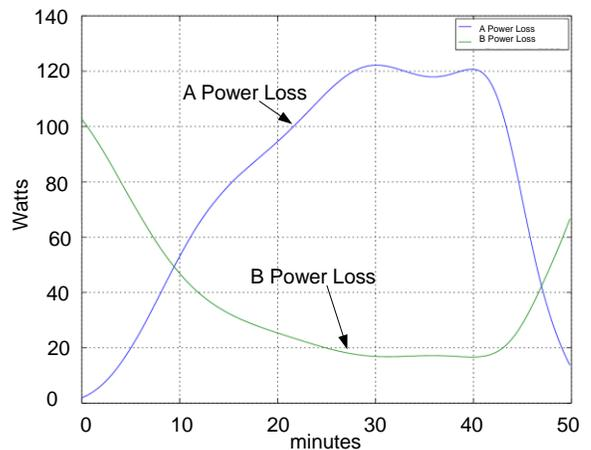
**Figure 6. A||B simulated power losses with a 120 Amps constant current load**
