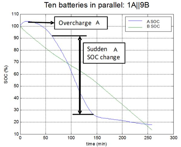
Figure 11. 1A||9B simulated SOC for each battery with a 120 Amps constant current load
