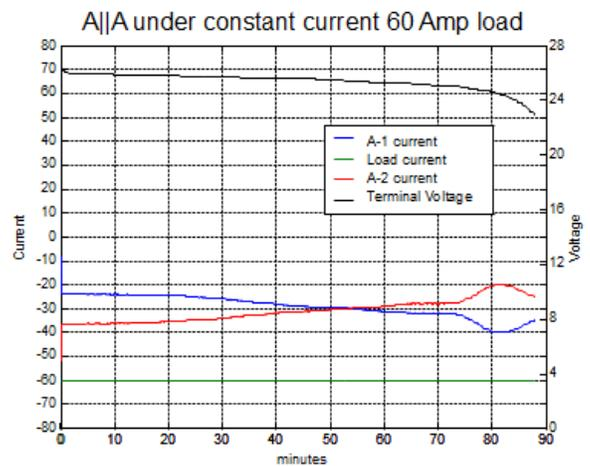
**Figure 12. A||A current and voltages under a constant 60 Amps load**
