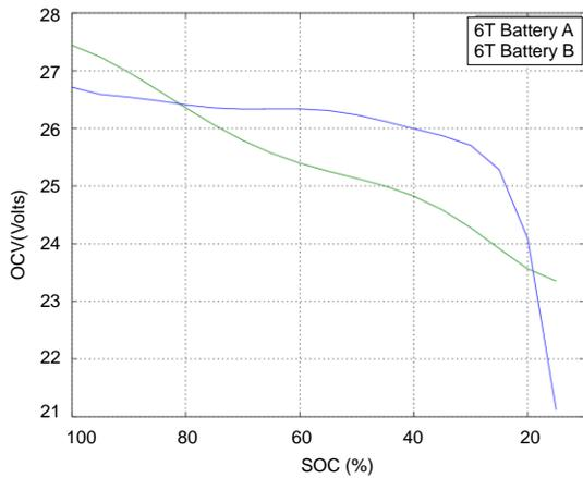
**Figure 2: OCV(SOC) of lithium-ion 6T battery packs A and B. Battery packs are of dissimilar chemistry**
