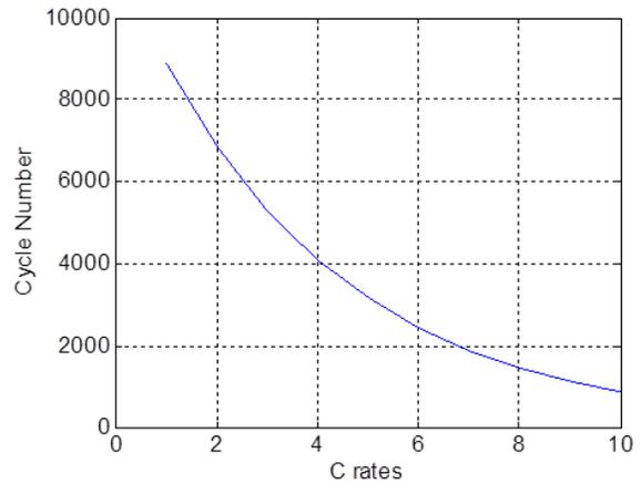
**Figure 19. Capacity fade in a  $\text{LiFePO}_4$  battery pack at different C rates. Temperature  $40^\circ\text{C}$  and DOD = 90%**
