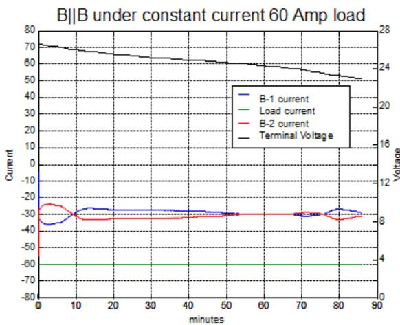
Figure 13. B||B current and voltages under a constant 60Amps load
