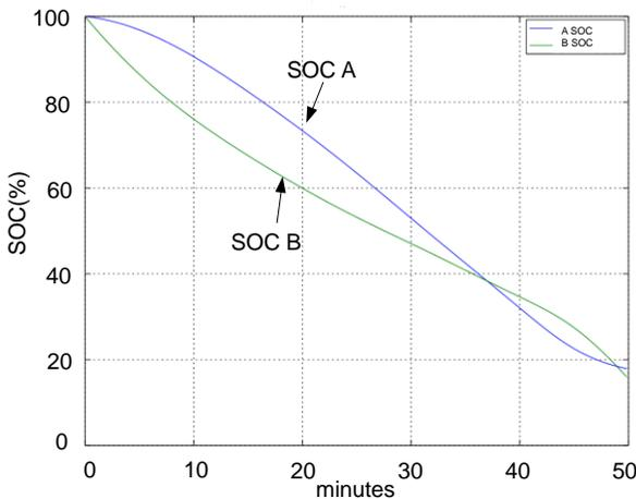
Figure 7. A||B simulated SOC for each battery with a 120Amps constant current load
