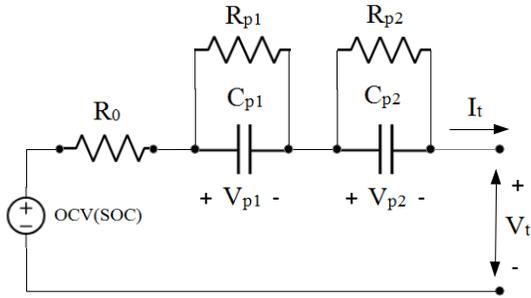
**Figure 1: Circuit Equivalent Model of a lithium-ion 6T battery pack**
