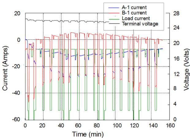
**Figure 17. Test of A||B under a constant current scaled silent watch profile**
