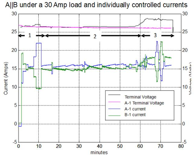
**Figure 21. A||B with individually controlled currents under a 30 Amps load. During segment 2 current is maintained approximately balanced in open loop**
