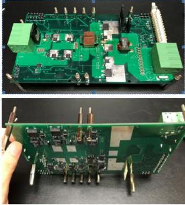
**Figure 20. GEN 1 Power converter prototype used for equalizing currents in parallel intermixing tests.**
