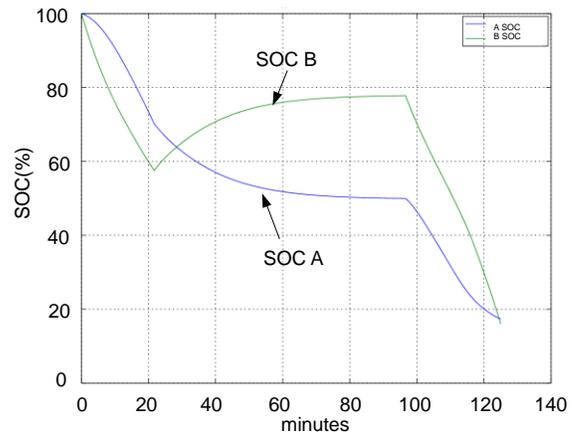
Figure 9. A||B simulated SOC with a 120 Amps constant current load interrupted
