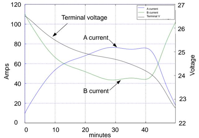
**Figure 5. Battery type A in parallel with Battery type B (denoted A||B). Simulated currents and terminal voltages with a 120 Amps constant current load**
