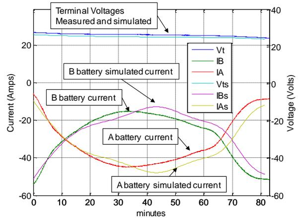
**Figure 4. Simulation and test of 6T Batteries A and B in parallel: A||B with a constant current discharge load of 60 Amps**
