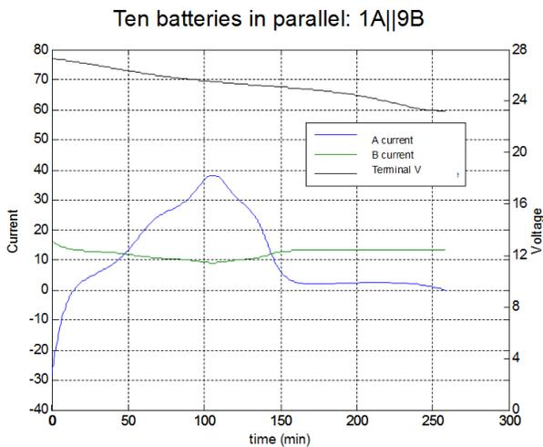
Figure 10. 1A||9B simulated currents and terminal voltages with a 120 Amps constant current load
