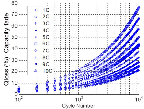
**Figure 18. Capacity fade in a  $\text{LiFePO}_4$  battery pack at different C rates. Temperature  $40^\circ\text{C}$  and DOD = 90%**
