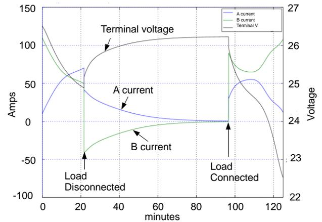
Figure 8. A||B simulated currents and terminal voltages with 120 Amps current load interrupted
