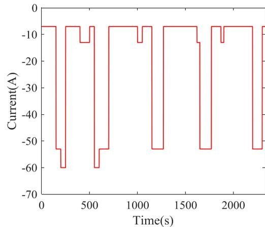
**Figure 15. Constant current scaled silent watch profile used for A||B test. A single period is shown**
