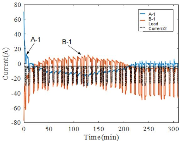
**Figure 16. Simulated A||B under a constant current scaled silent watch profile**
