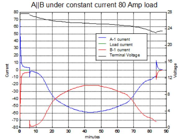
Figure 14. A||B current and voltages under constant load of 80 Amps
