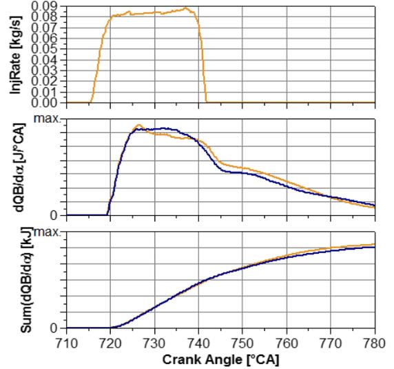
**Figure 5:** Injection rate as input and heat release results from 3D-CFD analysis at operating point 2
