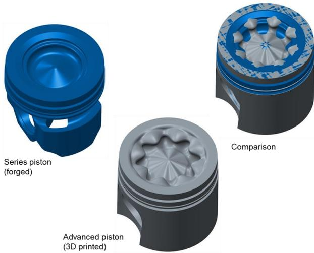
**Figure 2:** Comparison of a conventional and the advanced piston of IAV
