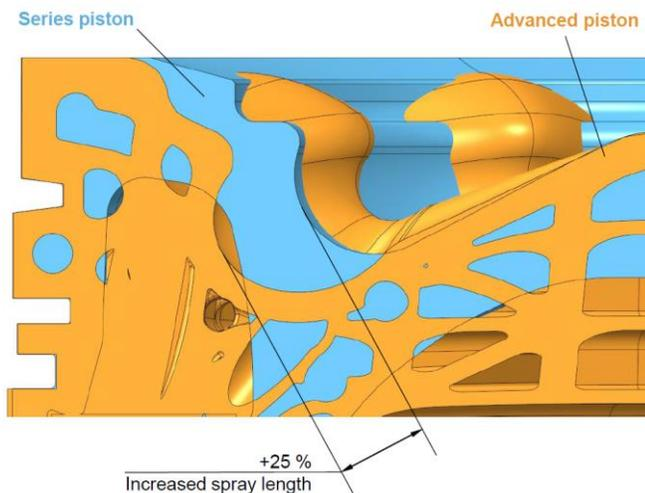
**Figure 3:** Longitudinal section through the conventional (blue) and advanced piston bowl (orange)
