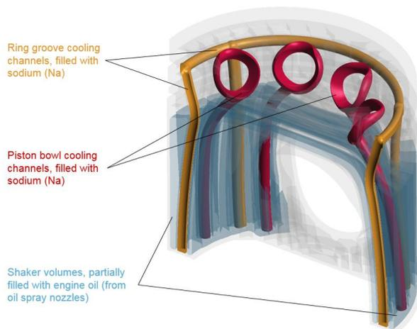
**Figure 7:** Two-stage cooling concept of the design study
