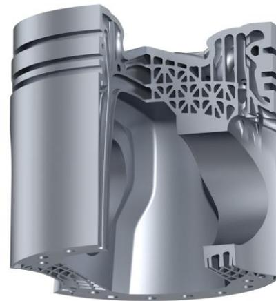
**Figure 8:** rib structure design of IAV
