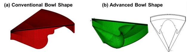
**Figure 4:** Numerical grids in top dead center position for 3D-CFD analysis
