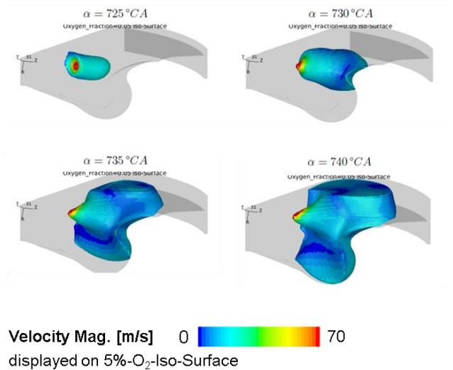
**Figure 6:** Visualization of combustion progress (result of 3D-CFD analysis)
