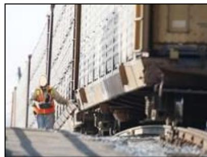
Figure 5: The conductor decoupling cars at the hump.
