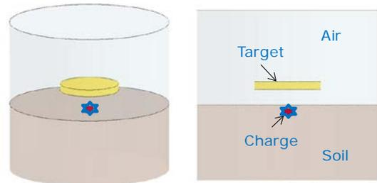
Figure 9 Rigid Plate Blast Model
