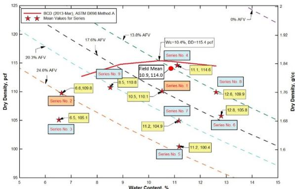
Figure 4 E-RW Soil Water Content - Dry Density Pairs Of Nine Test Series
