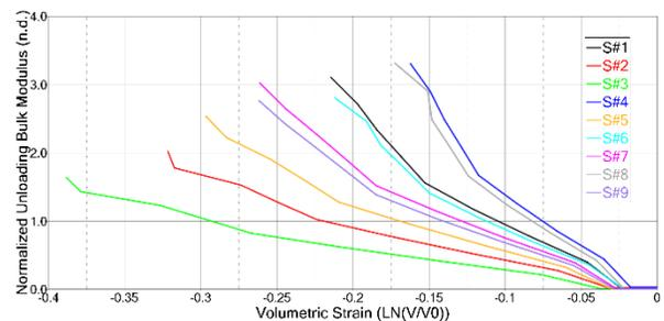
Figure 6 Bulk Unloading Modulus-Volume Relations for Nine Test Series
