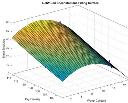
Figure 7 Fitting Surface of the Soil Shear Modulus
