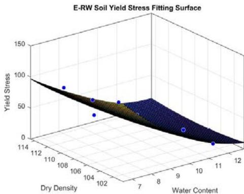
Figure 8 Fitting Surface of the Soil Yield Stress
