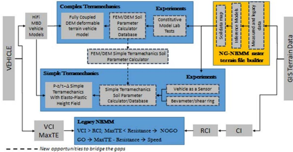
Figure 2: Replacing the Cone Index (CI) methods used in the current NRMM, simple Terramechanics models bring the full 3D mechanics of vehicles together with existing Terramechanics to provide a means for calculating critical mobility metrics on soft soil that are foundational components in the higher level mobility aggregated predictions of feasible trafficability (GO/NOGO regions) and maximum speed attainable.
