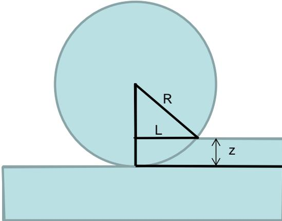
Figure 8: Example of a Contact patch calibrating length,  $L$ , estimation for a rolling wheel.
