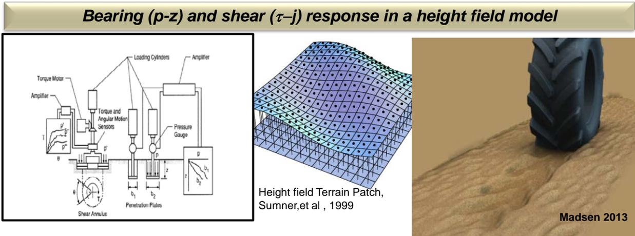
Figure 4: The classic Bekker-Wong-Janosi (BWJ) Terramechanics models (e.g., pressure-sinkage ( $p-z$ ), shear stress-shear displacement ( $\tau-j$ )), along with associated bevameter [4] experimental methods, are the most widely developed model suite that improves upon cone index approach and are ready for immediate application in NG-NRMM when implemented in the context of a terrain height field model [9- 13]
