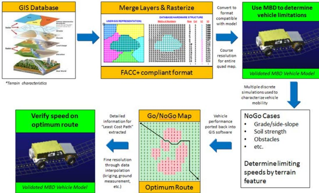
Figure 1: Full Featured NG-NRMM Simulation Begins with GIS based data, predicts mobility and maps it back onto the terrain as an additional GIS parameters[2]
