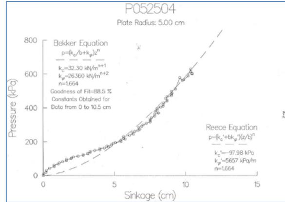
Figure 7: Pressure-sinkage data from a soil with an apparently weak top layer and loose deep under layer [24]
