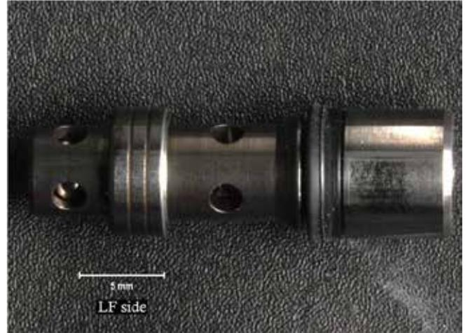
Figure 4. SBF front plunger. Pumping end (left), follower end (right).
