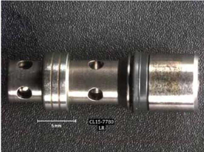
Figure 7. DOT III rear plunger. Pumping end (left), follower end (right).
