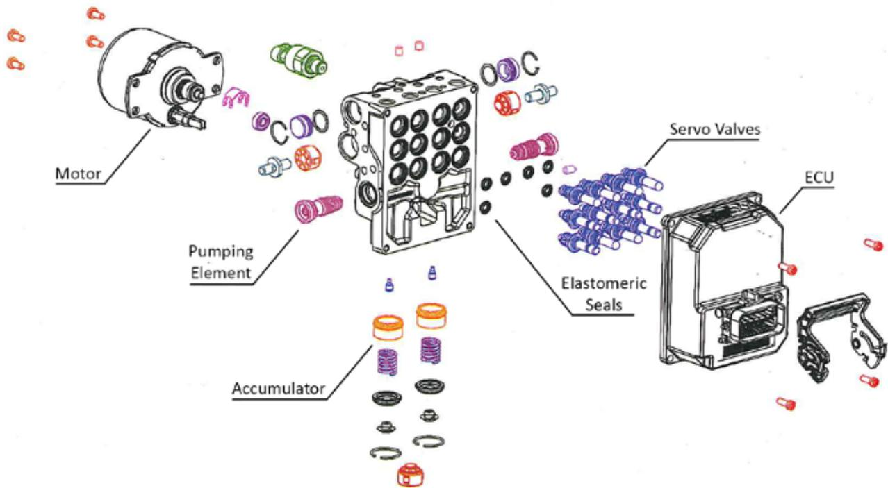
Figure 2. Detail view of ABS components. [7]
