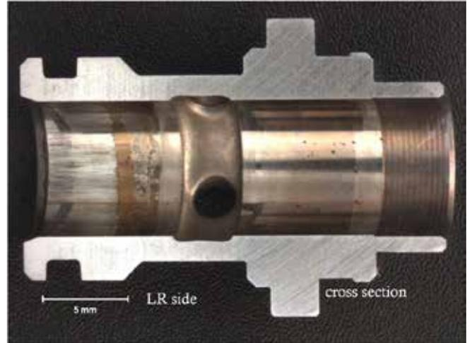
Figure 10. SBF rear plunger barrel cross section.
