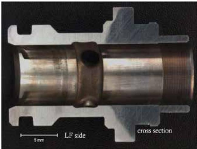
Figure 8. SBF front plunger barrel cross section.
