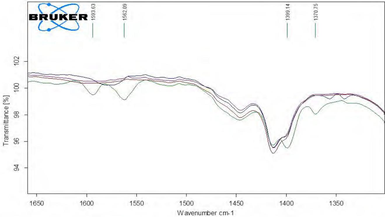
Figure 12. FTIR analysis of new and used SBF, as well as the solid residue from reservoir filter. Used SBF is identified as purple for the bottom layer, brown for the top layer. New SBF is identified as magenta. SBF reservoir residue is identified as green.
