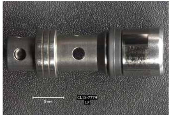
Figure 5. DOT III front plunger. Pumping end (left), follower end (right).
