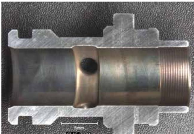
Figure 9. DOT III front plunger barrel cross section.
