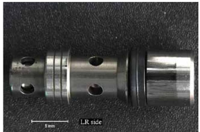
Figure 6. SBF rear plunger. Pumping end (left), follower end (right).
