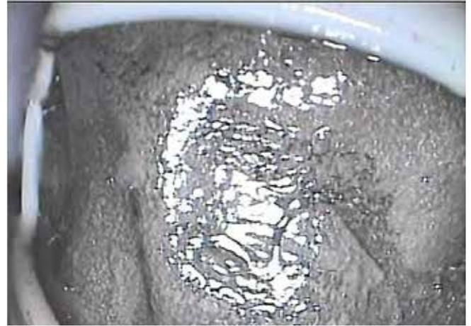
*Figure 3. Pumping filter inlet mesh screen after 20,000 pump and dump cycles with SBF.*
