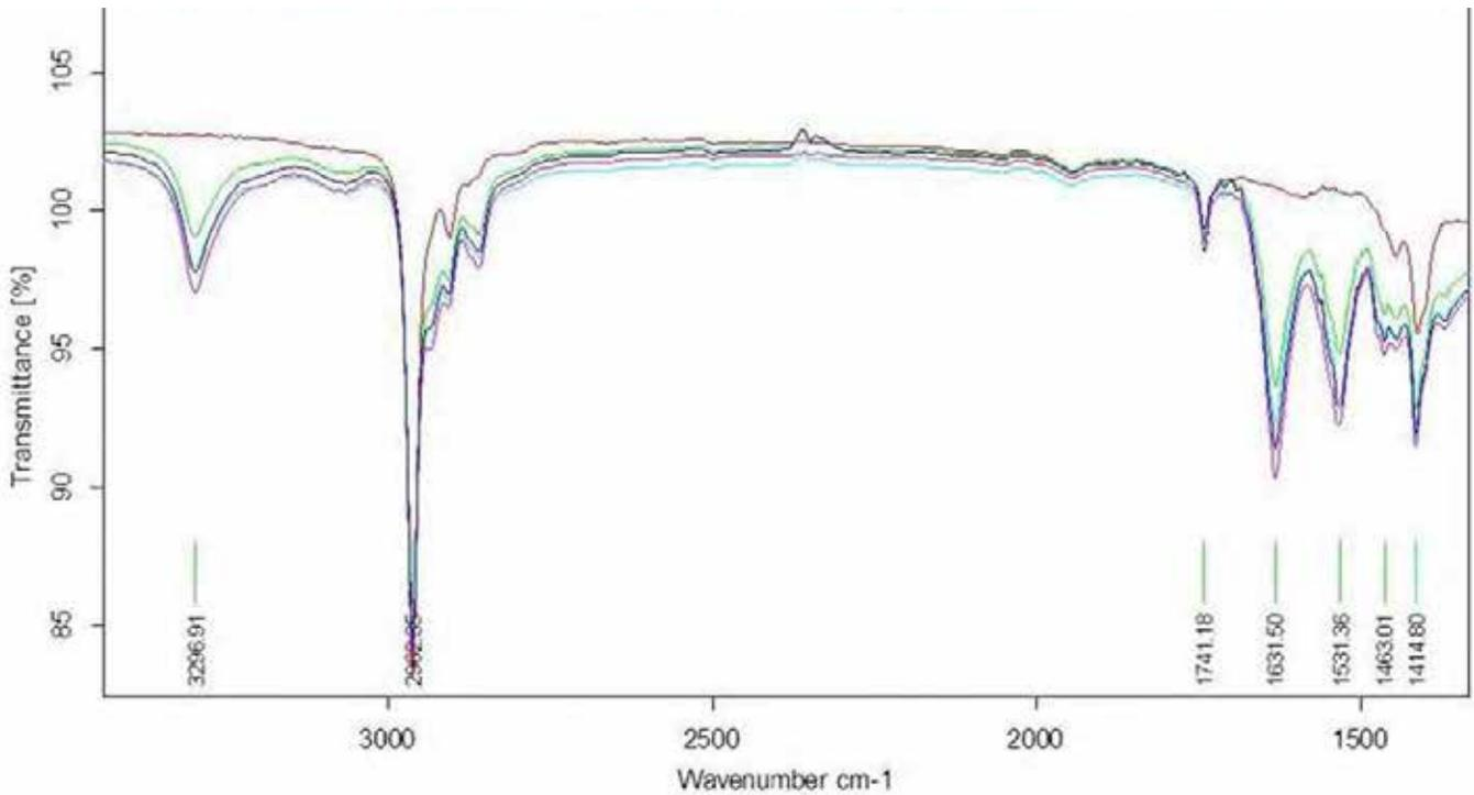
Figure 13. FTIR analysis of servo valve filters (No. 4 - purple, No. 5 - magenta, No. 6 - green, No. 10 - blue), and new SBF (brown).
