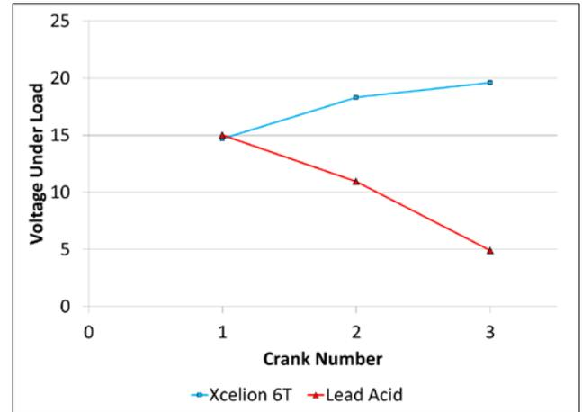
**Figure 5:** 400A/30sec pulse capability at -40°C
