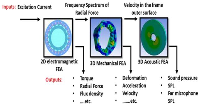
Figure 4: Structural simulation flow diagram.
