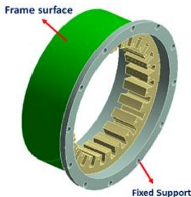
Figure 5: FEA SRM model for mechanical analysis.
