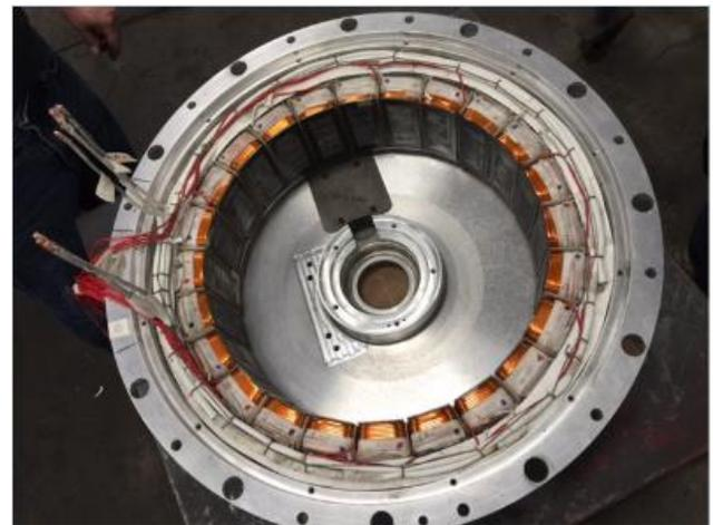
Figure 8: Stator development of the Windowed ISG.
