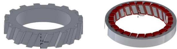
Figure 7: Skewing of SRM stator/rotor stacks.
