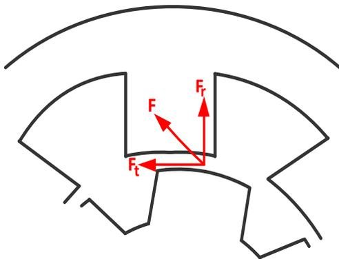
Figure 1: Magnetic force and its component.
