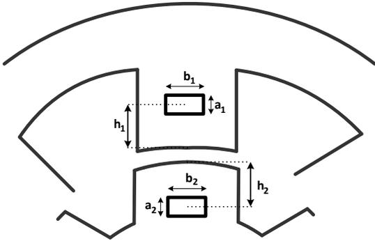
Figure 6: Stator/Rotor poles windowing of the SRM.
