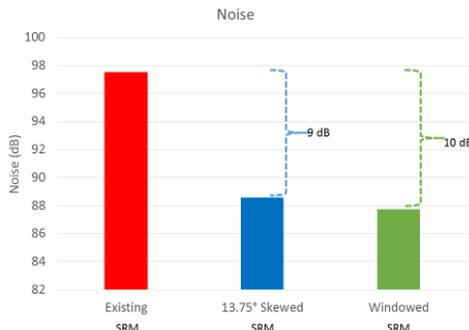
Figure 11: Weighted acoustic noise measures of the skewed, Windowed and the Baseline.
