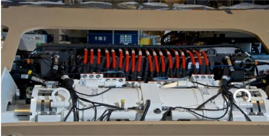
**Figure 8:** QinetiQ E-X-Drive® installed in the ‘Hot-buck’ SIL (Photo courtesy BAE Systems).
