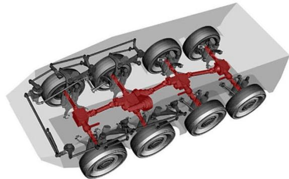
**Figure 2:** Boxer Multirole Armoured Vehicle (MRAV) (driveline highlighted in red). Photo courtesy UK Ministry of Defence (MOD).
