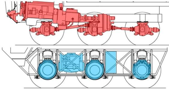
**Figure 3:** QinetiQ 6x6 powertrain comparison – conventional (red) vs. hybrid (blue).
