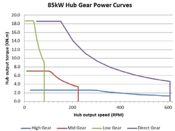
**Figure 10:** Hub drive torque-speed map (with hypothetical single-ratio direct-drive motor for comparison).
