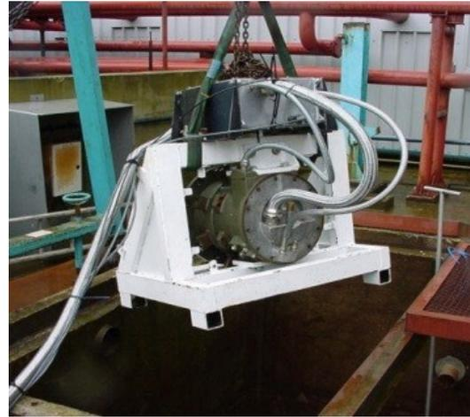
**Figure 15:** Immersion testing of earlier HDU
