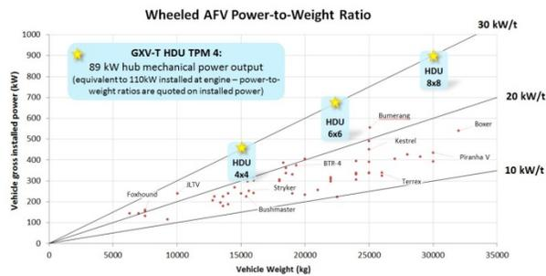
**Figure 9:** Chart of power-to-weight ratios with representative HDU installations indicated
