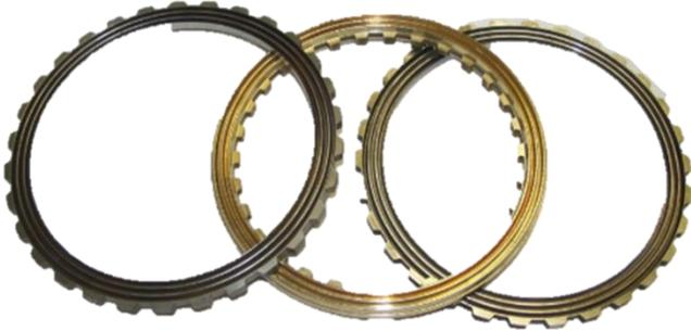
Figure 3 - PolyCone clutch pack assembly
