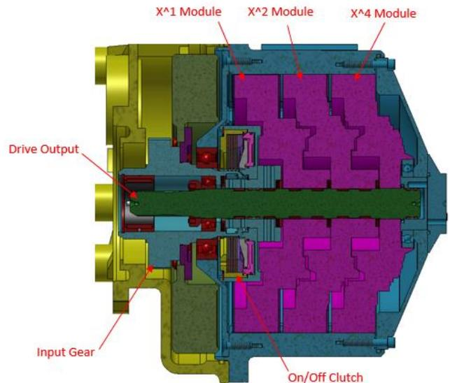
Figure 12 - Cross-section of the 8-Speed EPTO fan drive
