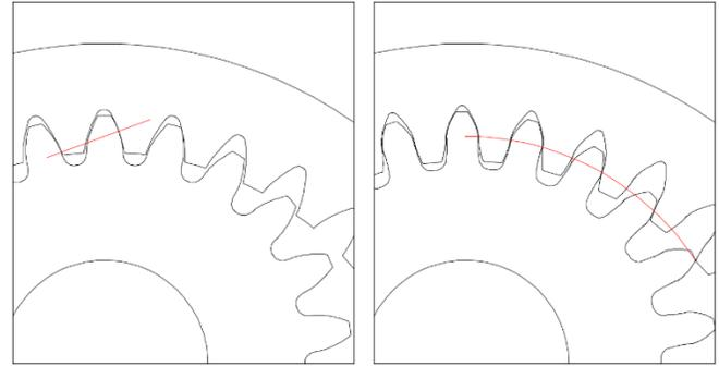
**Figure 1 - Paths of contact [Left-Involute tooth flanks; Right-Addendum-form tooth flanks]**
