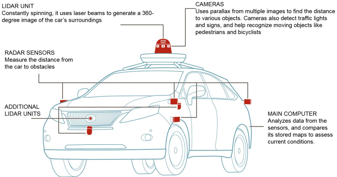
**Figure 2: How an Autonomous Vehicle Drives Itself**
