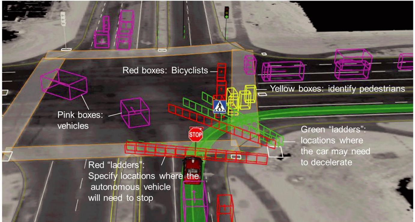
**Figure 3: Detection and Categorization of Typical Objects**
