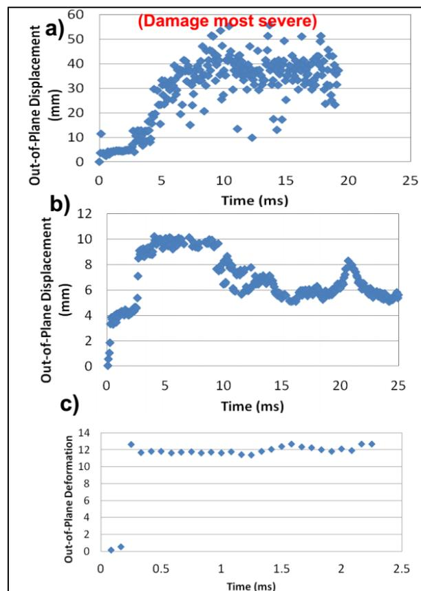
Figure 8 Out-of-plane displacement history as captured through fringe projection.
