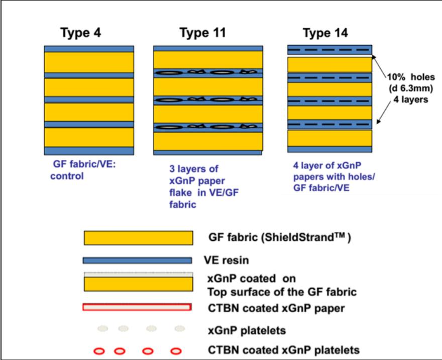
Figure 3 GnP-enhanced glass fiber reinforces vinyl ester composite construction types.
