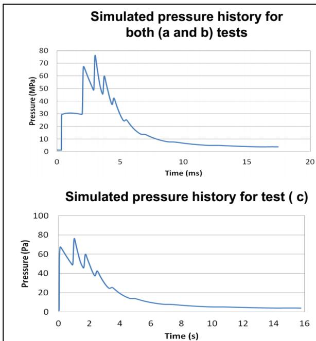
Figure 5 Simulated blast pressure histories.
