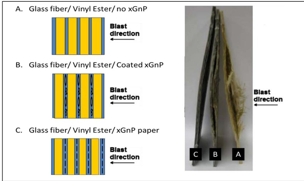
Figure 7 Edge-wise view of composite laminates following blast impact.
