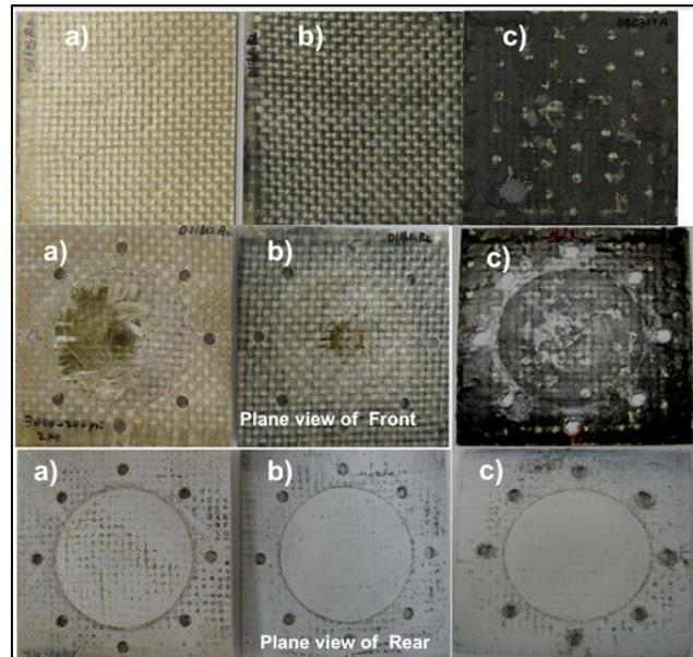
Figure 6 Views of composite laminates prior to and following blast testing.
