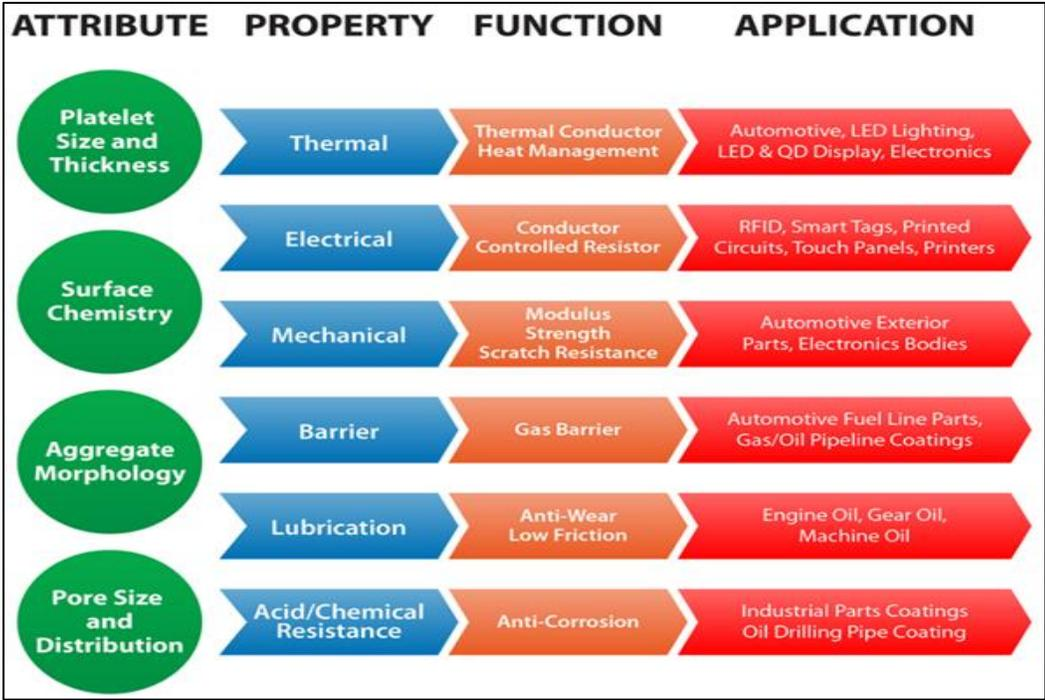
Figure 2 Graphene nanoplatelets: attributes, properties and example applications.
