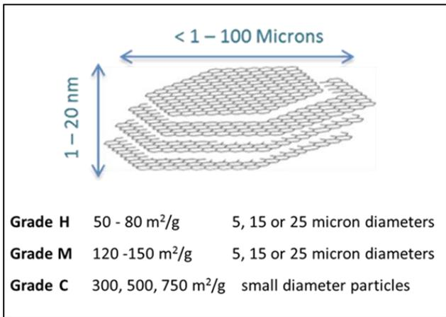
Figure 1 Graphene nanoplatelets.
