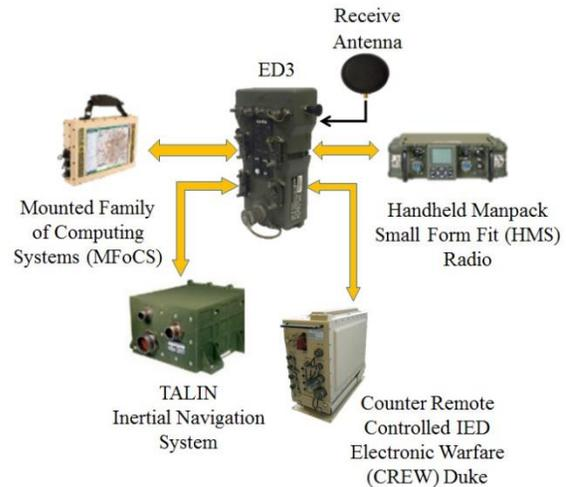
Figure 4 ED3 Notional Installation
