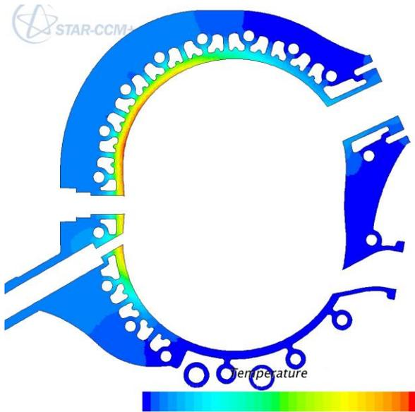
**Figure 2: R350 Metal Temperature Analysis**
