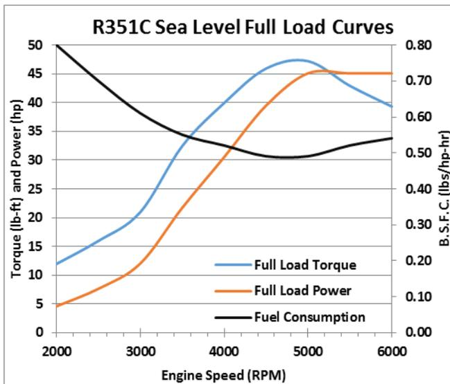
**Figure 9: Current R350C Power Curve and Fuel Consumption**
