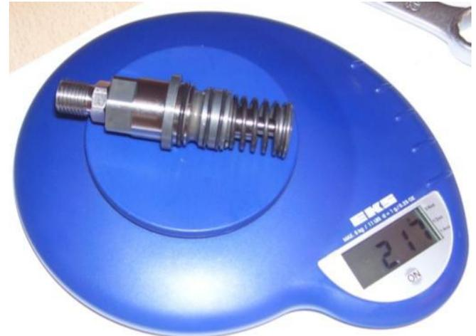
**Figure 1: High Pressure Fuel Pump**
