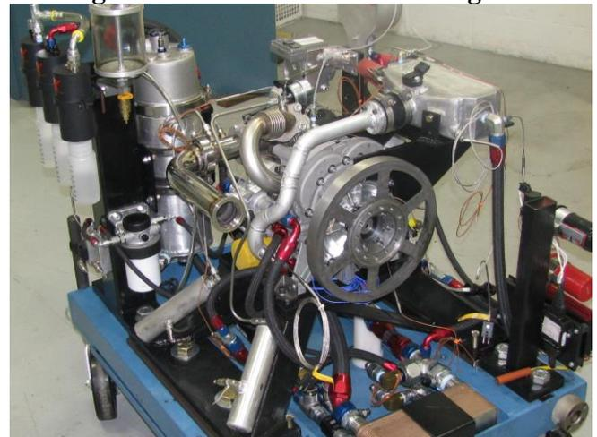
**Figure 6: R351 C-Series, Dyno Test Cart, Accessories and Instrumentation**
