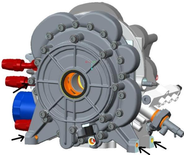
**Figure 4: Rear Cover and Bottom Mounting Locations**
