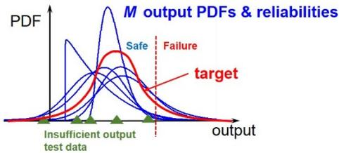
**Figure 1: Uncertainty in target output PDF and reliability due to insufficient output test data**
