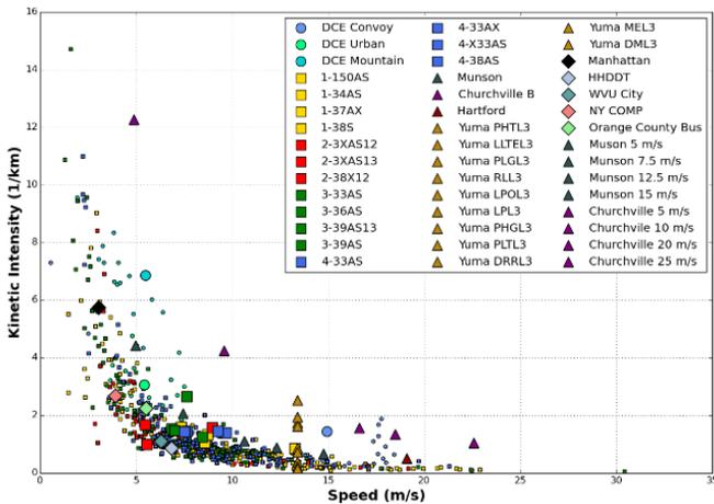
Figure 1. Average speed over the cycle versus the kinetic intensity for simulated cycles (circle), field cycles (squares), test cycles (triangles) and commercial cycles (diamonds)
