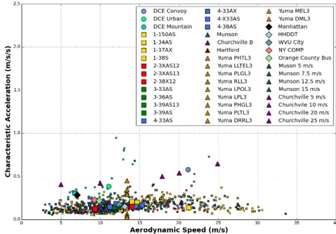
**Figure 5.** Characteristic acceleration versus aerodynamic speed for simulated cycles (circle), field cycles (squares), test cycles (triangles) and commercial cycles (diamonds)
