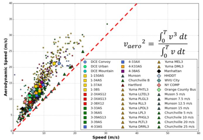
**Figure 6.** Aerodynamic speed versus cycle average speed for simulated cycles (circle), field cycles (squares), test cycles (triangles) and commercial cycles (diamonds). The 1:1 ratio is given by the red dashed line.
