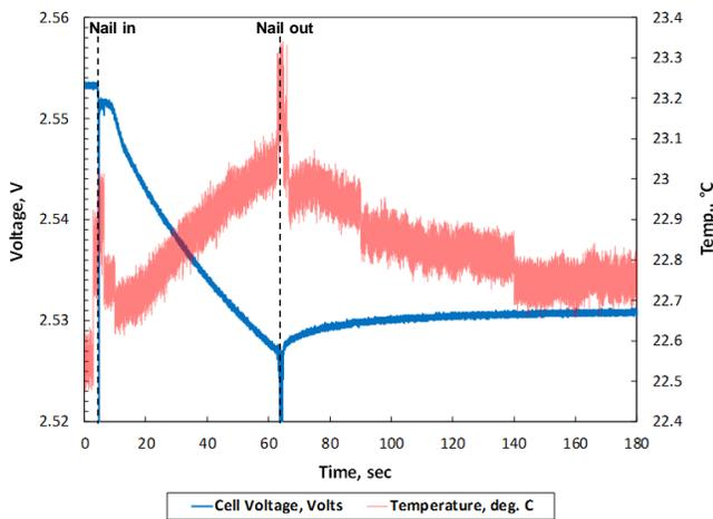
**Figure 5:** Voltage and surface temperature of a charged (2.65 V) 2.7 Ah CAM-7<sup>®</sup>/LTO pouch cell during penetration by a blunt 2 mm diameter nail at 1 cm/sec.
