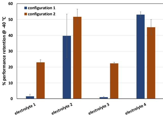
**Figure 11:** Retention of 1C, 30 sec. duration pulse discharge performance at -40 °C by unfixed 130 mAh CAM-7®/LTO pouch cells after storage in charged state at 78 °C (172 °F) for 40 days.
