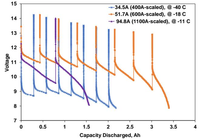
**Figure 8:** 600 A-scaled, 1100 A-scaled and 400 A-scaled 30 sec. pulse capacity delivered by 6 Ah module at -18 °C, -11 °C and -40 °C, respectively.
