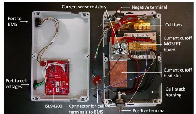
**Figure 6:** Photograph of 6-series-cell, 6 Ah module.
