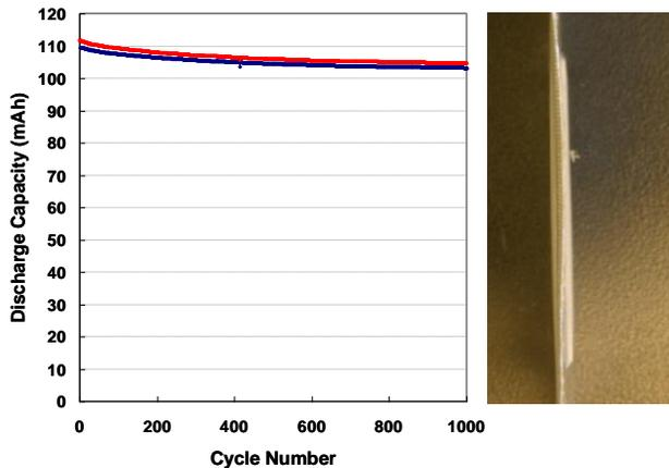
**Figure 3:** Left: Discharge capacity of 2 unfixed 120 mAh CAM-7®/LTO pouch cells cycled 1000 times between 2.43 V and 1.2 V at 10C/10C rate at 45 °C. Right: Side-on photograph of one cell after 45 °C cycling.
