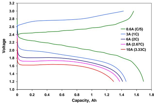
**Figure 2:** Constant current charge and discharge characteristics of a 3 Ah, 1.7 mAh/cm<sup>2</sup> loading CAM-7®/LTO pouch cell at -50 °C.
