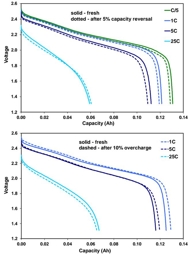
**Figure 10:** Constant current discharge at ambient temperature of unfixtured 130 mAh pouch cells before and after (top) 5% capacity reversal, and (bottom) 10% overcharge.
