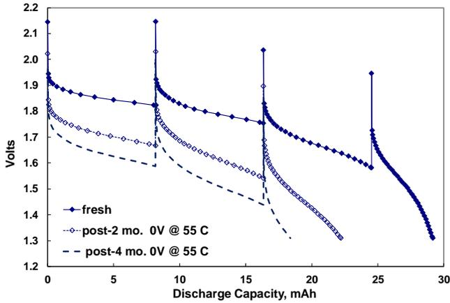
**Figure 9:** Repeated 0.93A, 30 sec. pulsing of an unfixtured 50 mAh CAM-7®/LTO pouch cell to 1.31V cutoff with 30 minutes rest between pulses at -18 °C, when the cell was fresh, after 2 months storage in 0 V condition at 55 °C, and after 4 months storage in 0V condition at 55 °C.
