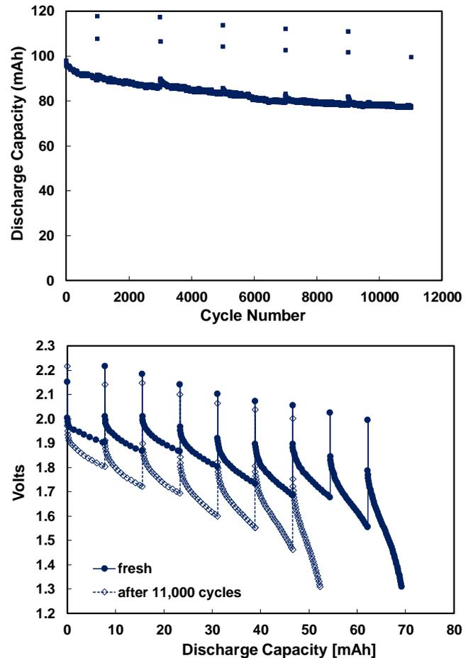
**Figure 4:** Top: Discharge capacity of an unfixed 120 mAh CAM-7®/LTO pouch cell 10C/10C cycled between 2.59 V and 1.31 V at ambient temperature, with C/5 and 1C cycles at 2,000 cycle intervals. Bottom: Capacity and voltage for repeated 0.93A, 30 sec. pulsing of the cell to 1.31V cutoff with 30 min. rest between pulses at -18 °C.
