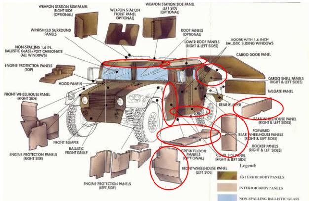
**Figure 12:** Selected non-hinged armor of an M1100 HMMWV that might accommodate a structural battery.
