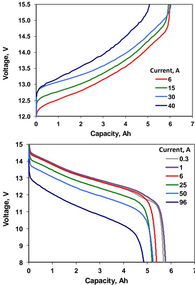
**Figure 7:** Constant current charge (top) and discharge (bottom) characteristics of 6-series-cell, 6 Ah module.
