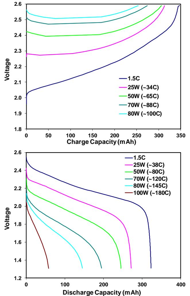
**Figure 1:** Continuous constant power charge (top) and discharge (bottom) characteristics of a 320 mAh, 0.5 mAh/cm<sup>2</sup> loading CAM-7®/LTO pouch cell at ambient temperature.
